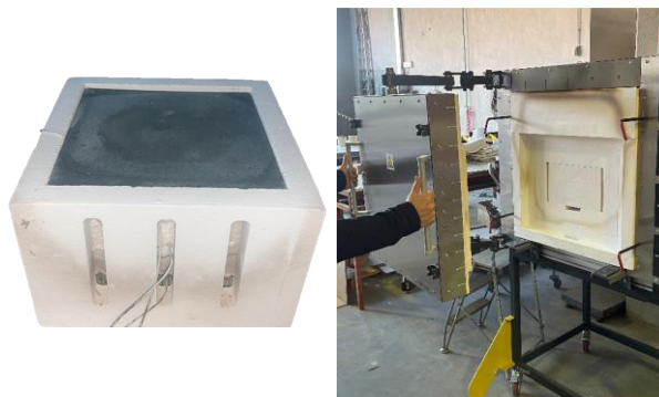
Fig 20. Insulation stack-up set-up and test furnace
