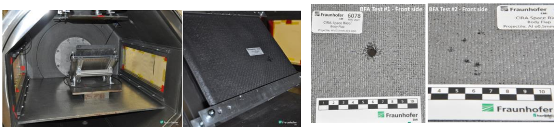
Fig 18. BFA scaled model within Space Gun Test Facility, test #1 sphere dia; 2.3mm V = 6,5 km/s – and test #2 5 spheres dia 0,5; mm V = 4,9 km/s
