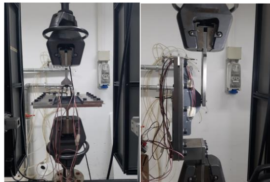
Fig 19. Tensile test and shear Y set-ups
