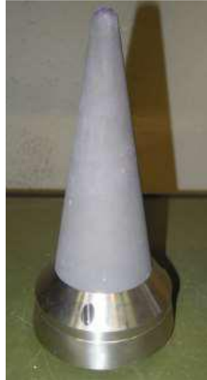
Fig 3. Metallic substrate Sharp cone and wedge and CMC substrate wedge after coatings
