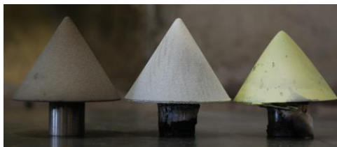
Fig 10. Conical samples uncoated and coated with different coatings
