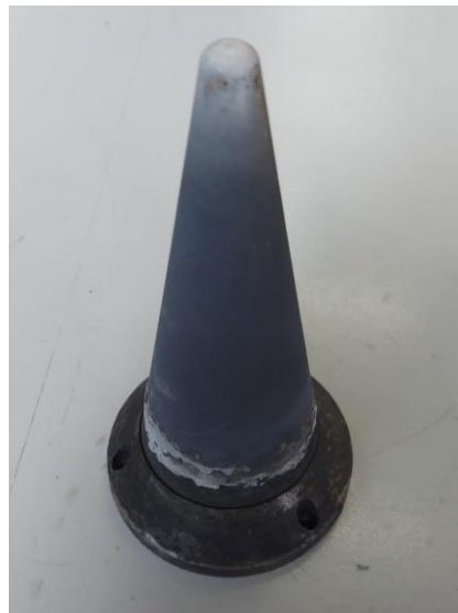
Fig 19. Post-tests Blunt cone appearance
