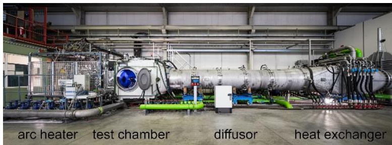
Figure 12: Arc-Heated Wind Tunnel L3K [14]
