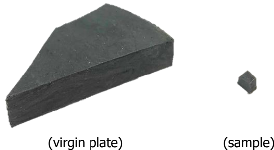
Fig. 2 Picture of the plate and the virgin samples used for the TGA
