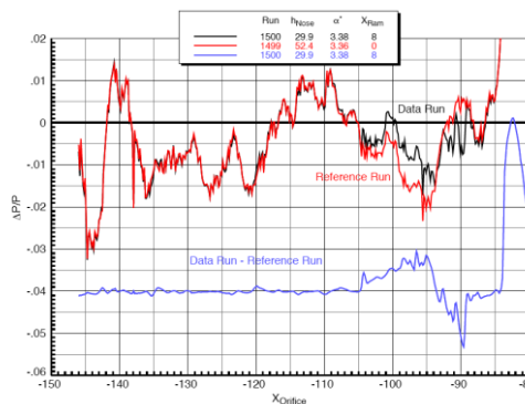
Fig. 6 Isolate model pressure signature from rail by reference experiment technique (ref. 1)
