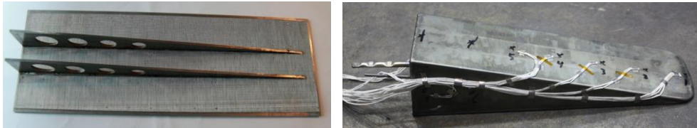
Fig 2. Structure of wedge-shaped high-temperature heat pipe.
