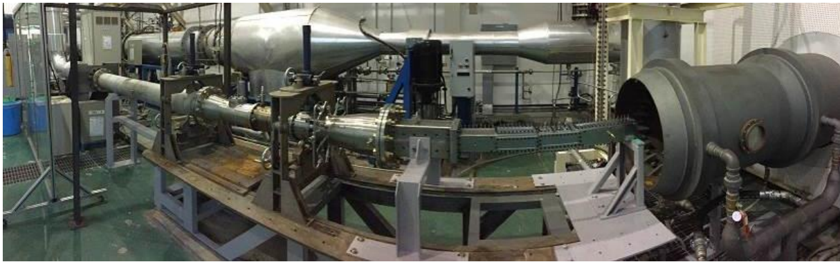
Fig 3. Direct-connected supersonic combustor test facility
