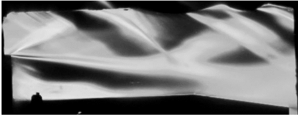
Fig. 14 The structure of the flow of burning hydrogen in the air flow in the path with a deformed body
