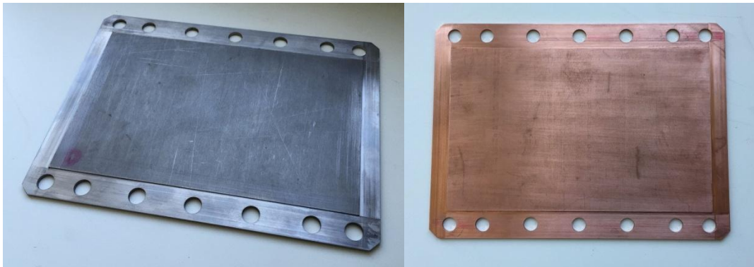
Fig. 5. VT20 and M1 copper test plates
