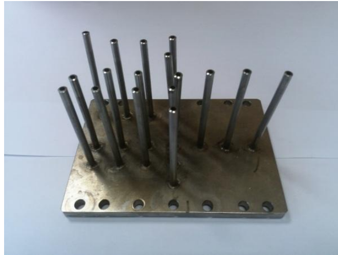
Fig. 9. Stainless steel dummy plate with 10 mm pressure probes
