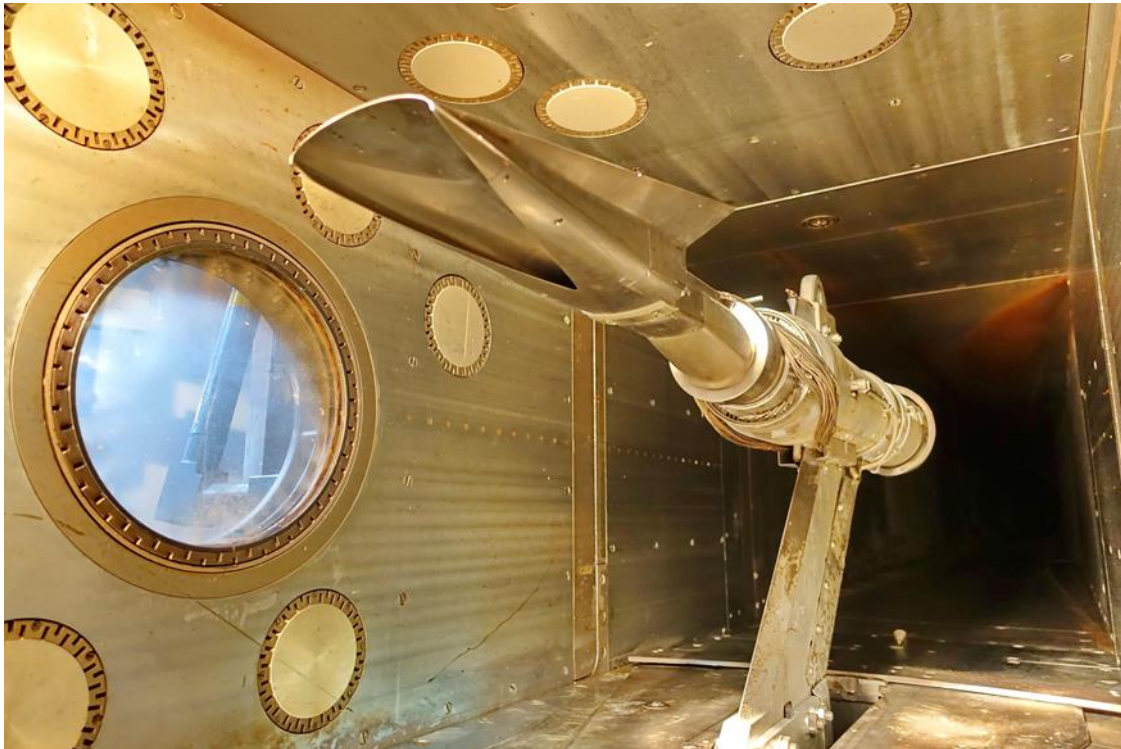
Fig. 3 Intake model testing in WT T-116 TsAGI
