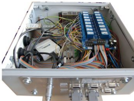
Fig. 3. Test bench for time resolved resistance measurement
