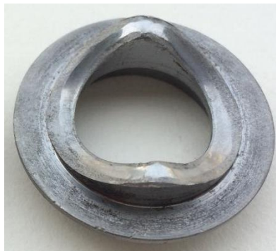
Fig.3 Image of a spatial cam
