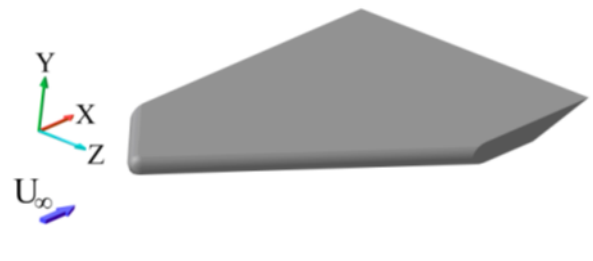
Fig. 1b. 3D picture of 60% model of the wing with a sweep angle 55^\circ
