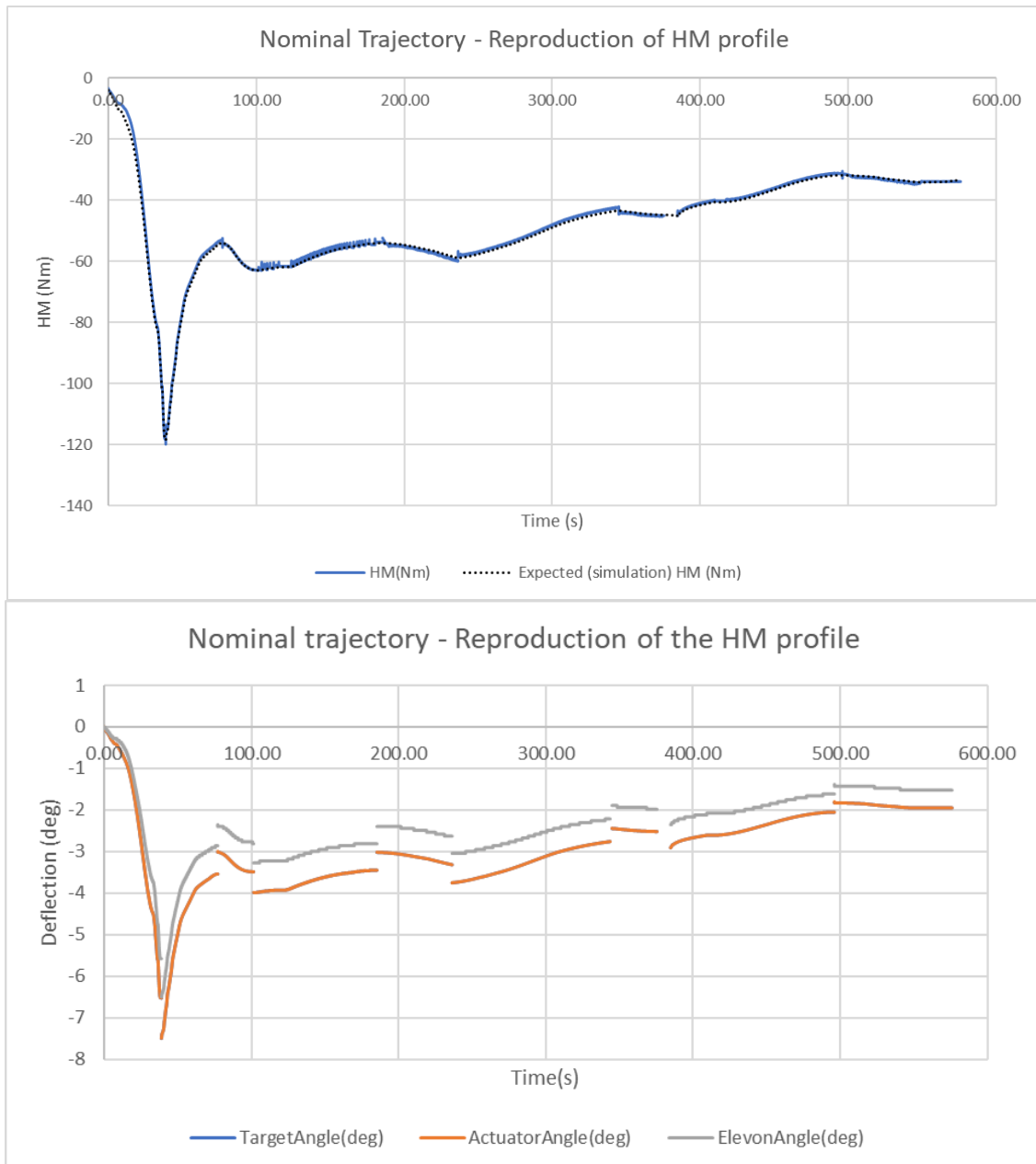
Fig. 17: Reproduction of the nominal trajectory HM profile by parts (top) and required deflections to reproduce the nominal's trajectory HM profile by parts (bottom).
