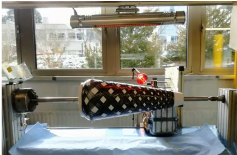
Fig. 12. Manufacturing of the TPS segment B in the CFRP initial status via filament winding.
