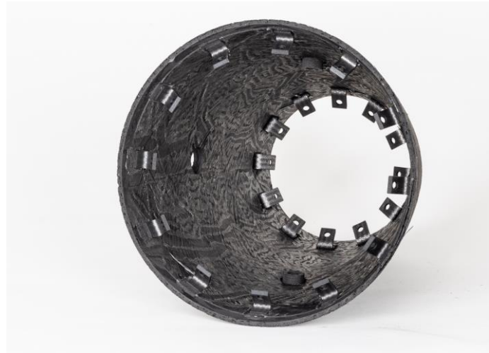
b) Segment B after the joining of all connection elements
