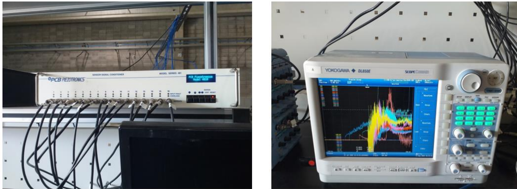
Fig 2. Signal conditioner (left) and oscilloscope (right).
