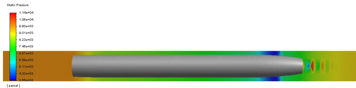
Figure 15. Static Pressure contour ( M=0.6 , \beta = 0.36 , P=10 kPa)
