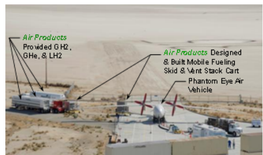
Figure 17: Air Products liquid hydrogen tanker truck and the fueling of the Boeing Phantom Eye liquid hydrogen-fueled aircraft.
