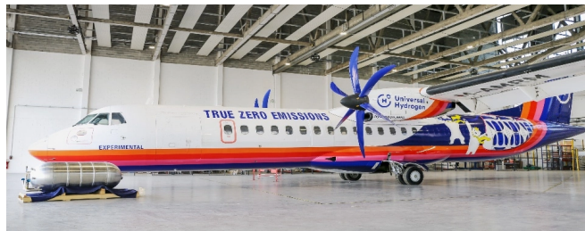
Figure 14: ATR72-600 next to the retrofit tank [24].
