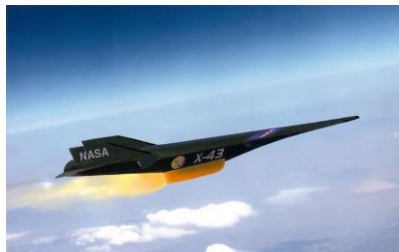
Fig. 1. NASA X-43A Pegasus scramjet-powered vehicle which reached M = 9.6 [1]
