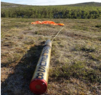
Fig 13. Microgravity experiment section MAPHEUS 8 with integrated hybrid module after ground impact
