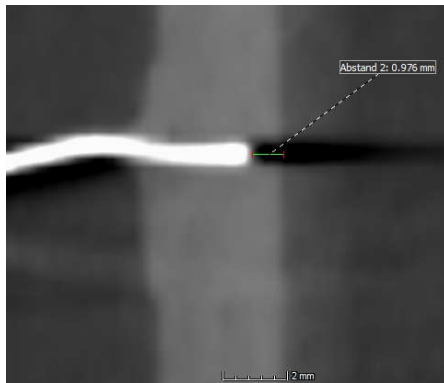
Fig 4. CT of mounted Thermocouple
