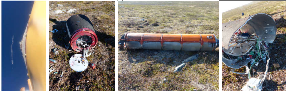
Fig 17. Loss of Fins, view from \mu g-Payload (left), Motor Adapter after impact (middle-left), S-30 Motor after Impact (middle-right), Tailcan after Impact (right)
