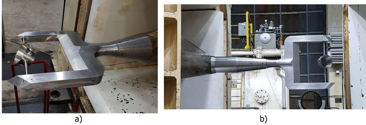
Fig. 2 FTT model installed on the rig, a) roll angle 0 deg, b) roll angle 90 deg
