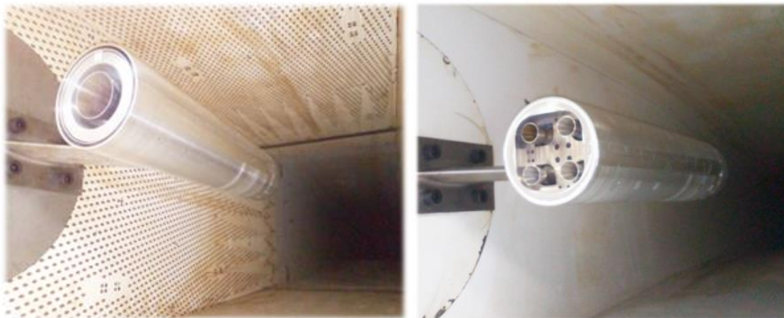
Fig. 6 - Model mounted perforated and solid walls test section
