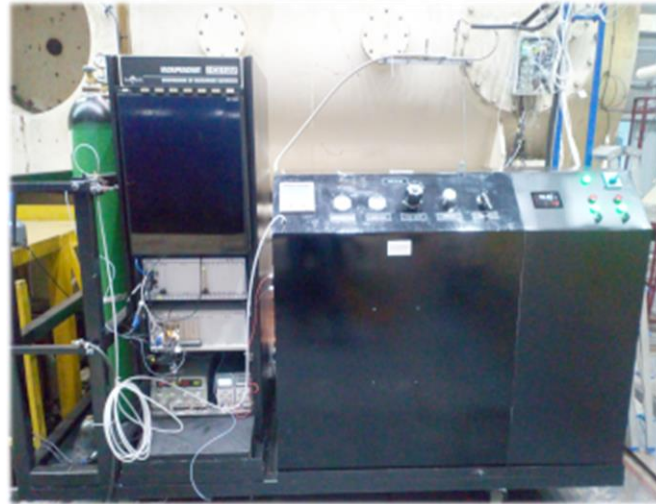
Fig. 2 - Engine supply system
