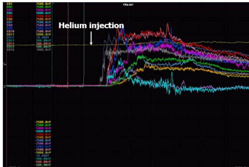
Fig 10. Evidence of He injection during the test time of the experiment, with a pressure of P_i = 3.5 bar being injected.
