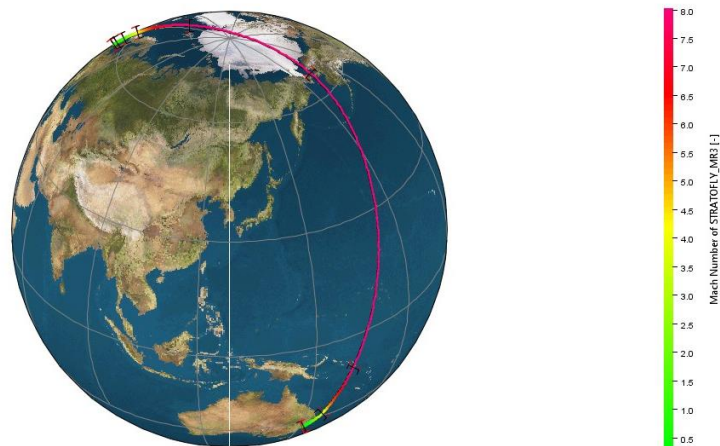
Fig 4. Overview of complete trajectory BRU-SYD. Trajectory characterized by Mach number.
