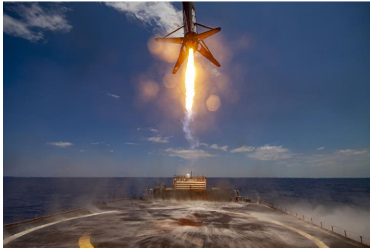
Fig 1. SpaceX Falcon 9 stage landing on a barge (Photo by SpaceX ; CC BY-NC 2.0)
