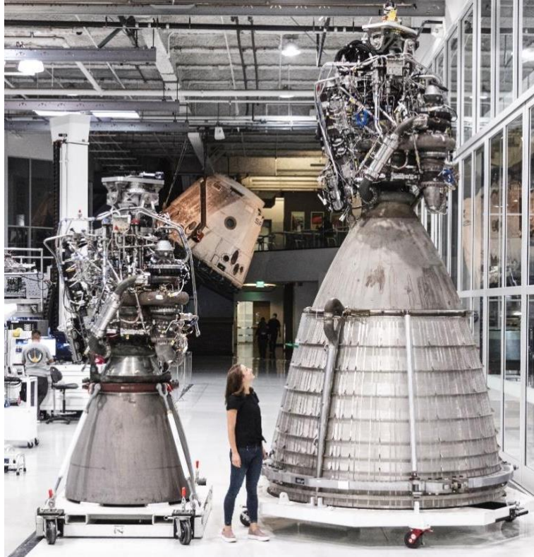
Fig 1. SpaceX Raptor engine with booster type (left) and upper stage (right), from [4]
