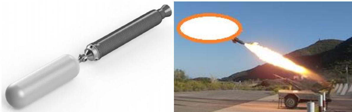
Fig 10. N 2 O-paraffin hybrid RATO booster: rendering (left), flight (right)
