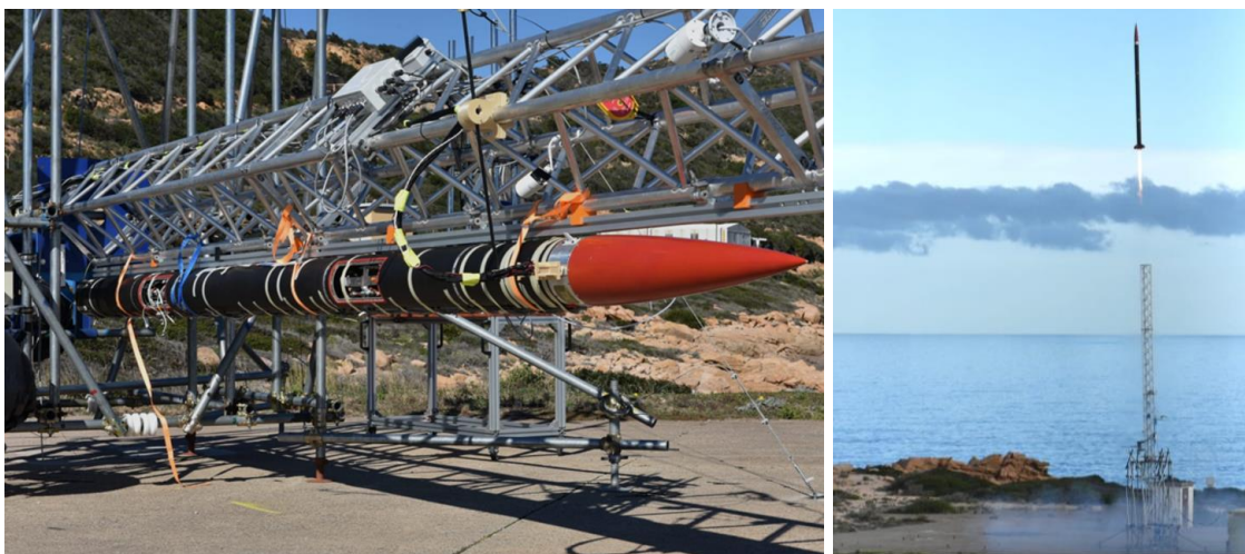
Fig 14. H 2 O 2 sounding rocket: on the ramp (left), at launch (right)
