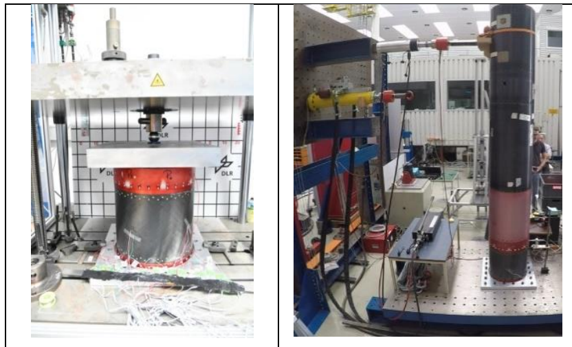
Fig 7: Mechanical tests (left) and bending test (right) on hybrid module
