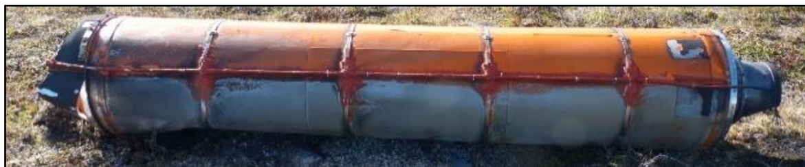
Fig 17: Second stage (S30 motor) after ground impact
