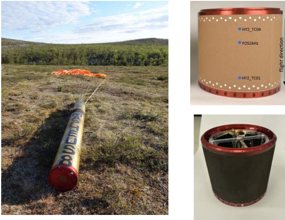
Fig 13: Microgravity experiment section MAPHEUS 8 with integrated hybrid module after ground impact (left) and Hybrid module before and after (right) the flight
