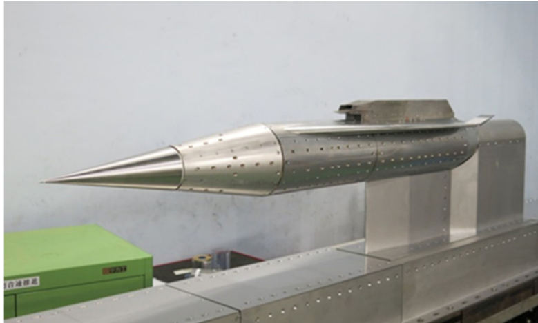
Fig. 1. Wind tunnel test model of High Mach Integrated Control experimental aircraft
