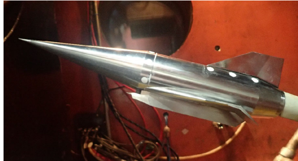
Fig. 6. HIMICO-#1 wing tunnel test model
