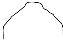
Fig 14. An ablated graphite nose-tip, in a transitional flow regime (redrawn from Ref. [44]).
